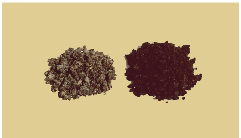
Effect of water on binder coating. Sample on the right contains adhesion promoter
